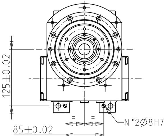
Two dowel holes can be drilled in the table feet, as indicated in Fig. 4. The two holes allow precise positioning and make the table interchangeable.
