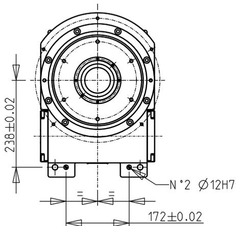
Two dowel holes can be drilled in the table feet, as indicated in Fig. 8. The two holes allow precise positioning and make the table interchangeable.
