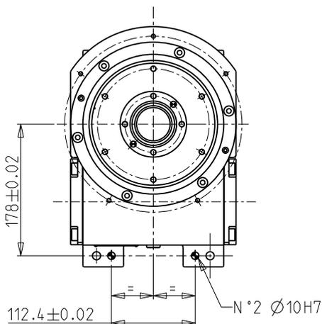
Two dowel holes can be drilled in the table feet, as indicated in Fig. 6. The two holes allow precise positioning and make the table interchangeable.
